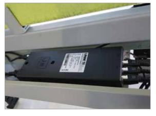
A small and compact microprocessor control box is used to translate the signals from controller into perfectly controlled movement. It is available in 2 main versions, a 2-channel version (200W) and a 2, 3 or 4-channel version (300W) with more effect.
